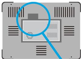
1. The power supply is located at the bottom of the Dreamer. Gently rest the Dreamer with the front panel facing down. Hold the extruder set while doing this. You will see the power supply switch.
