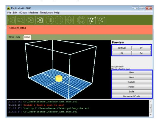
When the object is imported you may find that it is not on the virtual build platform or even on the screen, using the function keys indicated by the blue boxes in the illustration above, you can change the camera angle and reposition the object onto the center of the build platform. Once you've done this, the next step is to generate the Gcode. This is achieved by clicking on the button (Generate GCode) at the bottom of the panel.
