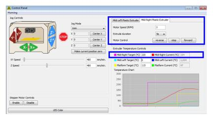
To heat the right extruder and feed material, click the right extruder on the upper right corner of the control panel and manually modify the temperature in the "Right Target" setting for the extruder temperature control changing the temperature to 220°C. A red line will be plotted in the temperature map. When the actual (Current) temperature reaches 220°C you can pull the filament out.
