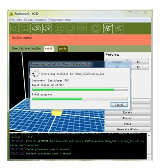
After the Gcode is generated, the temperature of the bottom plate needs to be changed if you print PLA filament. See below for the required modification. First, select Gcode as shown highlighted in the illustration below and change M109 S110 to M109 S50 to set the HBP temperature at 50°C. Then click File > Save to save this modification. If you print ABS filament, then no HBP temperature modification is needed.
