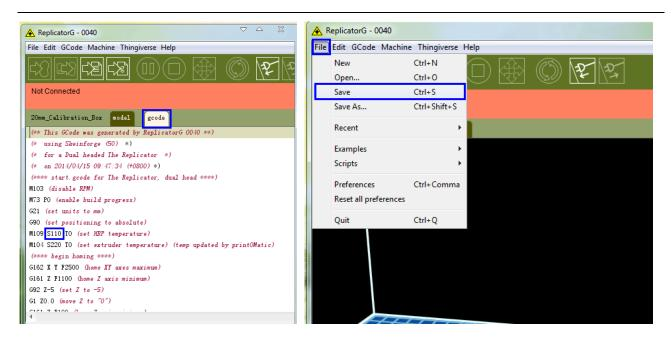
If you have connected Replicator G Creator Pro printer, click the left most button on the green bar near the top of the screen. The Gcode has now been sent to the printer and the object will start printing shortly. If not, please refer to <a href="USB Connection">USB Connection & Temperature Setting</a> to connect.
