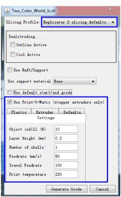
If you want to print dual colors with ABS filament, select Replicator slicing defaults under the Slicing Profile column, and lower the Feedrate to 60 and Travel Feedrate to 80.
