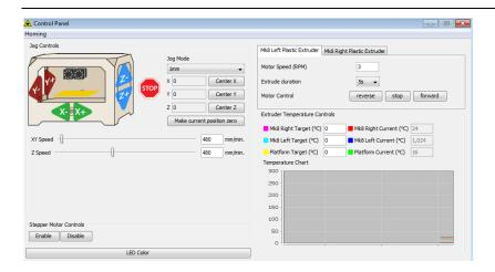
Input the following target values: 220°C for the extruder and 115°C for the heating platform. After entering the values, the platform will start to warm up. When the extruder temperature reaches 50°C, the cooling fan will be activated and the current temperature value will display to the right as shown below.
