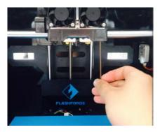
Install the side fan duct. To do this, find the side fan duct and attach it onto the left side of the extruder set. Secure it with the supplied M3x8 screw.
