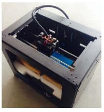
The build platform should now be visible. It is an aluminum plate covered in a thin polyamide film. This is the surface that your objects will be printed on. *Note:* Remember not remove the film.
