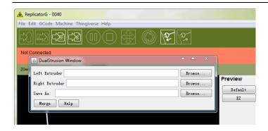
Click on the first Browse button to locate and select the file for left extruder; and then click on the second Browse button for right extruder. For example, you can find the examples folder in its installation path. Open the folder examples select Two\_color\_world\_a.stl for left extruder and repeat the process for the right extruder as shown below:
