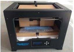
Now, open the accessory box and remove the accessory sleeve. You will find the dual extruder heads in the protective packaging along with the black cable, carefully remove it and place it on your work surface. Remove the cardboard packing material and take the accessory box from the printer, set it aside for later.
