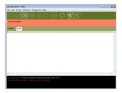
After opening ReplicatorG software, click on Machine to select your Machine Type. Choose The Replicator Dual for Creator Pro dual extruder machine.
