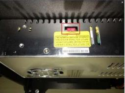
To do this, begin by carefully placing the Creator Pro on one of its sides so that the bottom is exposed. You will see the Creator Pro's power supply. Using a flathead screwdriver switch the red power supply switch so that it displays 115v, as shown below. Now you are ready to install the extruder.
