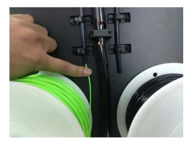
There are two ways of feeding the filament into the extruder head, one is using the LCD screen on the printer itself and the other is by using the control panel on the Replicator G software.
